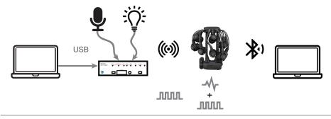
Computer running E-Prime or SuperLab is wired to the StimTrigger with a USB cable. Microphone and Light Sensor wired to StimTrigger. StimTrigger sends trigger data to CGX headset using CGX's patented low-latency wireless protocol. CGX headset combines EEG and trigger data into a single file, precisely combining trigger and EEG data, then sending it wirelessly to the recording computer.
