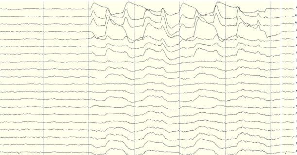
Moving the eyes will generate muscle artifact in the forehead and front of the head. A high concentration of neurons in the eyes generate strong electromagnetic fields, so eye movement causes disruptions in the EEG recording.
