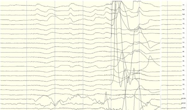
Excess or quick movement of the head may disrupt connection between sensors and scalp causing data artifacts as shown.
