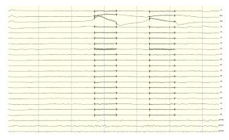
If the ground has poor contact, all channels will be impacted. Avoid disrupting the connection of the Ground electrode during use.
