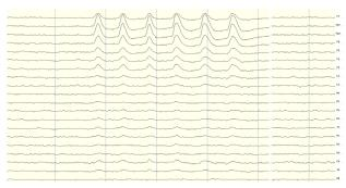
Eye blinks will generate muscle artifacts in the frontopolar locations (Fp1 and Fp2) and less so in frontal sensors (F3/F4, F7/F8), overshadowing brain activity in EEG recordings.
