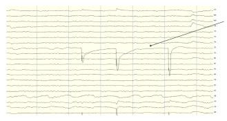
Brief disruptions in contact between sensor and scalp may cause "sensor pops" on recordings. Occasional pops can usually be ignored in processing, but if the problem persists, check the contact between the sensor and scalp.
