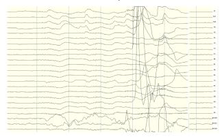
Excess or quick movement of the head may disrupt connection between sensors and scalp causing data artifacts as shown.
