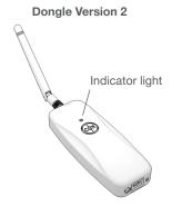
Green Idling Purple Searching For Device Blue Device Found Flashing Blue Data Transmission
